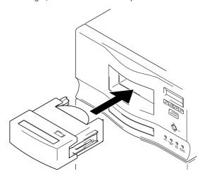
When the hyper magazine has been loaded, a unique magazine ID will be displayed together with the record of the locking mechanism.
